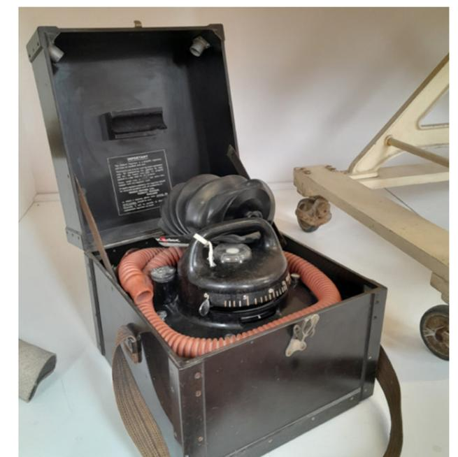
Figure 3: The Oxford Vaporiser, portable anaesthetic machine still being used by the British Forces during the Falklands War.
